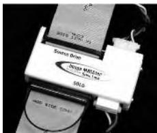
**Figure 3.2** Drive Lock. (Reprinted with permission, 2002.)
